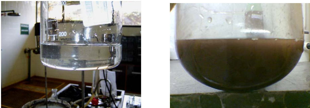
Fig. 8: Filtrate clarity - Ceramec® filter (left) and RVDF (right)
