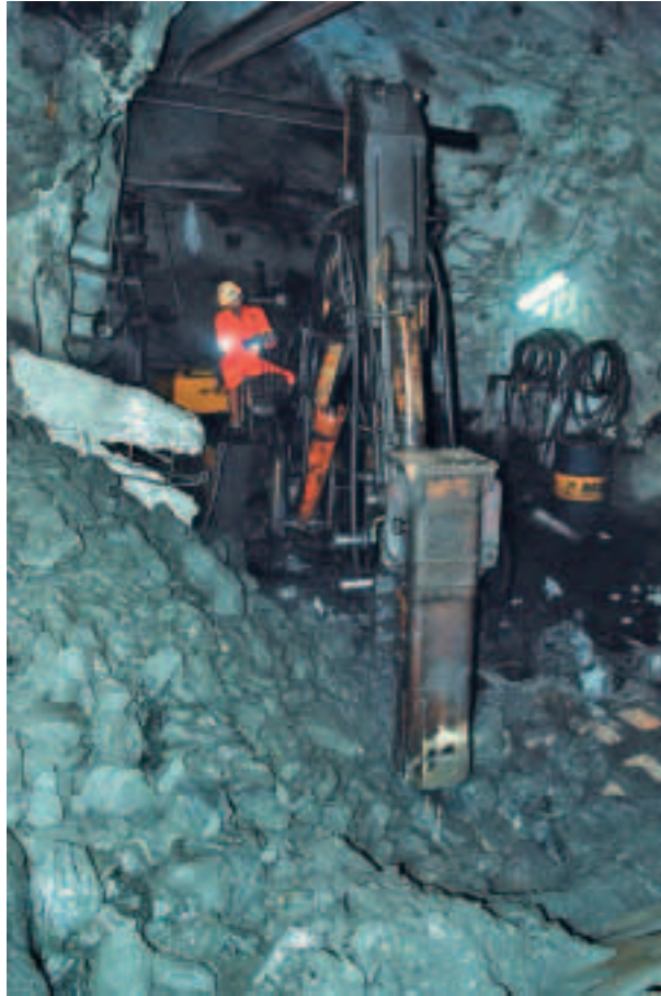
Breaking oversize rocks at Surda mine
