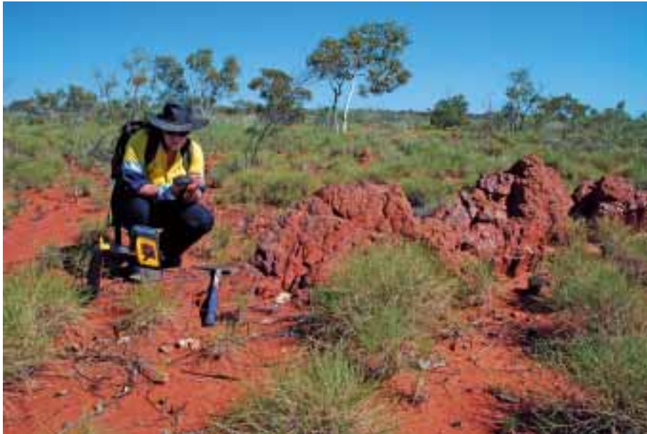
Innov-X Delta testing rock outcrop incorporating the Explorer GIS/GPS feature that allows instantaneous geochemical mapping in the field
