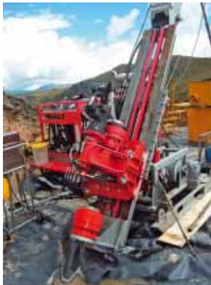
An Ingetrol Explorer 1500 rig, valued both for depth ability but also portability
