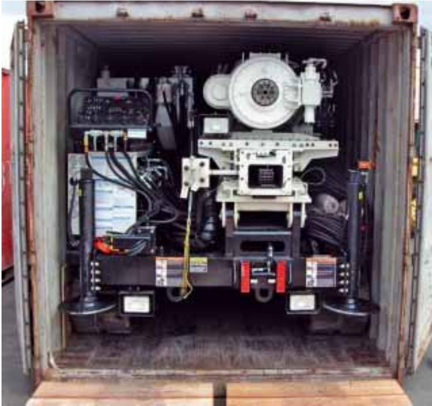
The Sonic Drill SDC-350 inside a 20 ft ocean container
