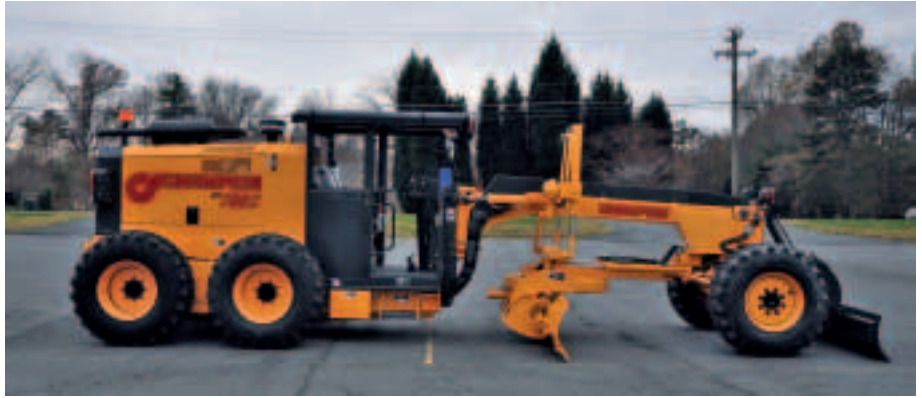
The Champion M786 C Mine Grader is only 2.13 m high and was completely designed from the bottom up to meet underground requirements
